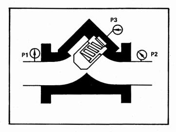
50% Open: The pressure differential across the valve (P1 minus P2) is equal to the spring force in the 50% open position.
